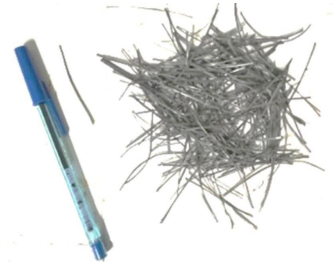
Figure 2: Synthetic polypropylene macrofiber used in the study
