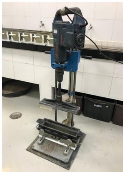
Figure 3: Vibratory compaction equipment to prismatic samples
